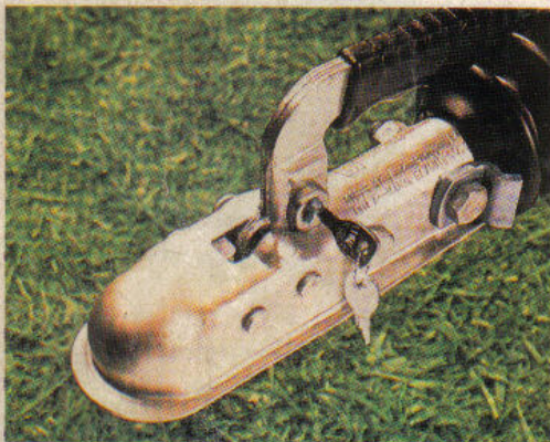
Key and locking device for additional security
