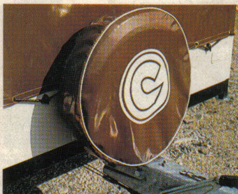
Spare wheel and cover with bracket for Braked and Unbraked models
