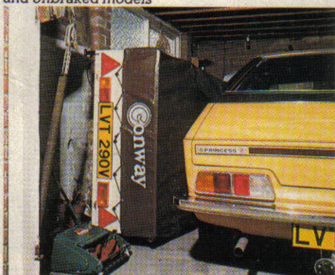
Steel framed castored storage brackets, enable you to manoeuvre the trailer through narrow side passages, etc.
