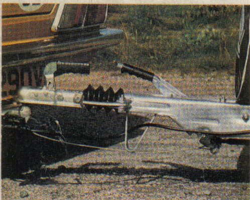
Inertia braking system recommended for use with small cars.
