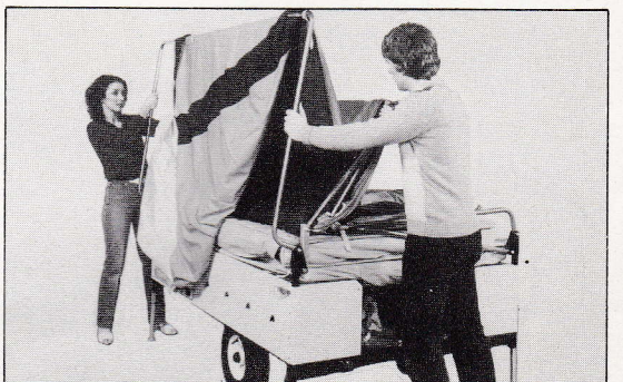
6. Swing over left hand cabin roof support frames and then same on right hand side.
