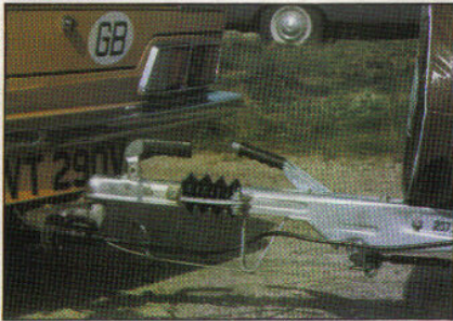
Inertia braking system recommended for use with small cars
