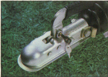
Key and locking device for additional security
