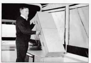
Lift over kitchen unit, arrange dinette cushions, clip up inner tents and roof liner. Reverse procedure to close trailer.
