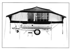
Connect five roof poles to front frame, fit the two other front legs and raise to full height. Tension roof poles and guy out.
