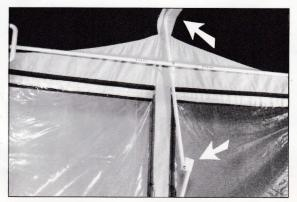
Step inside trailer making sure the centre roof ridge pole is central on double roof canvas strip then straighten ridge frame upright by closing the bracket.
