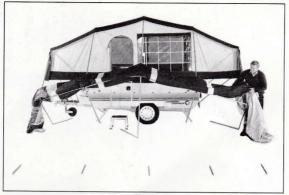
Fit two inner legs and centre leg to front frame. Take canvas from bag and lay out over roof poles.
