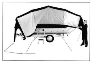
Connect straight front centre pole to right hand side leg assembly and feed through canvas sleeve.
