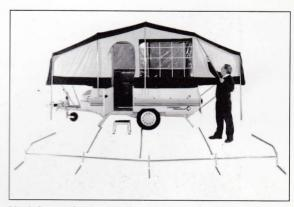
Hook five roof poles into holes in trailer frame through gussets in the canvas.
