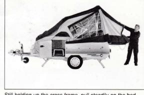
Still holding up the cross frame, pull steadily on the bed handle, slide bed out fully until it hits the end stops, the frame will automatically raise the cabin canvas.
