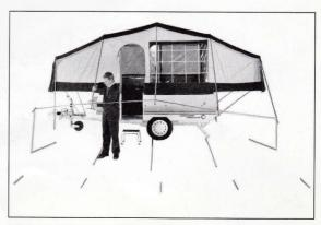
Lift front awning frame and connect the five roof poles with front legs "broken".
