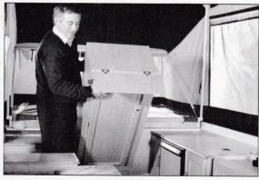
Lift over wardrobe and slide onto locker top. Locate four bed stop pins into holes in bed runner slides.
