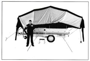
Connect left hand leg assembly to centre pole. Ensure eyelets are located over corner spikes.
