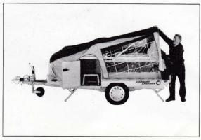
Standing at the back of the trailer, lift up the top cross frame and work up and down a few times. This allows air to get under the canvas enabling smooth slide out of the bed frames.
