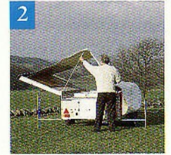
2 Turn Bed 1. over which lifts roof.
