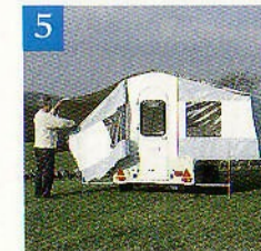
5 Lift the four Corners into place.
