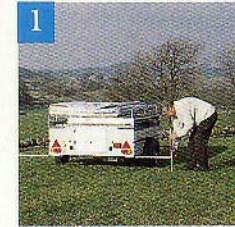
1 Level Trailer using Jockey Wheel (only adjustment required).
