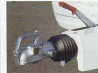
Triplelock security coupling head
