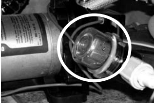
Fig. 8.3 Water pump strainer
