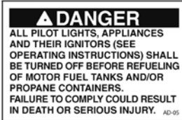
Fig. 7.3 “Shut off during re-fueling” label
