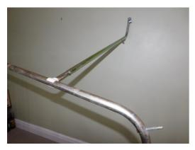
These poles then run along the inside of the annex canvas, into the awning (where the side panel would, normally, zip on). They then bend upwards and clip onto the outer roof tensioner pole in the main awning, using adjustable metal C clips.
