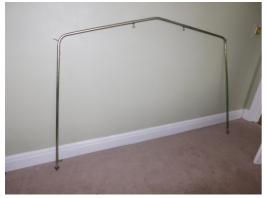
(2) Once we have assembled the rear roof section, we can add the two legs, which just slot in and lock into place, using a push button fixing.
