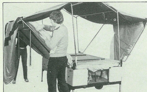
9. Fold over each bed board and mattress to each side. Check that each bed leg is securely located and adjust as necessary.
