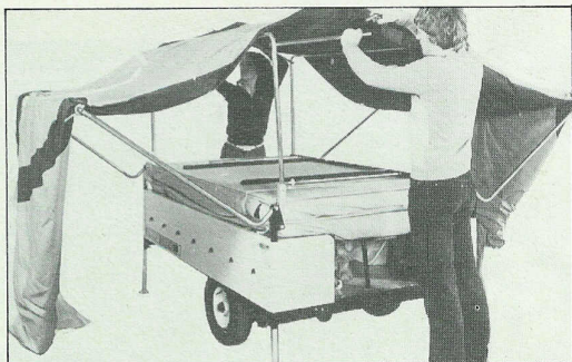
7. Lift up the two hinged arms to form the 5th roof support pole.
