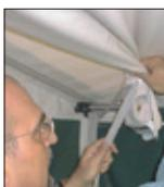
The frame's adjusters are tightened and the loose hanging sun canopy is tightened to the trailer body canvas by using the ribbons.
