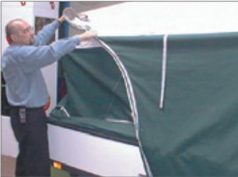
When closing the trailer down, to save time you may leave the sun canopy attached and stored on top of the trailer roof.
