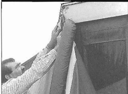
27. Remove the awning canvas from its bag and slide the white corded section through the awning channelling fitted to the camper roof.
