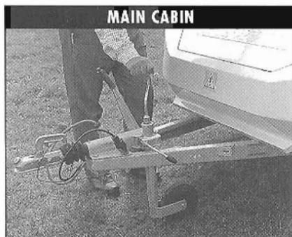
**1.** Apply handbrake and detach trailer from the car. Ensure trailer is as level as possible using adjustment in the jockey wheel. On uneven ground aid levelling by using wooden blocks or other aids beneath the wheels.
