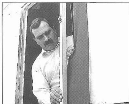
**21.** Release door catches and step inside the trailer, secure the plate at the top of the door with the white plastic turn buckles. Fit the canvas to the door by turning the hard edge through 180 degrees and pressing firmly into the door channel.
