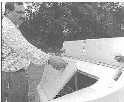
**2.** Unlock and lift the bottle box lid. Remove the corner steady brace handle, plywood pads and any other items required. Ensure the gas regulator is fitted and turned on.
