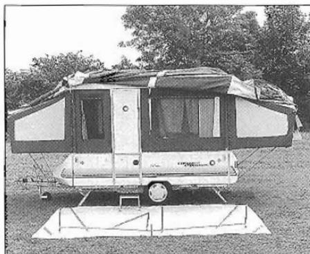
31. Layout the awning frame as shown, connecting together all sprung sections. See the parts list drawing for a more detailed diagram.
