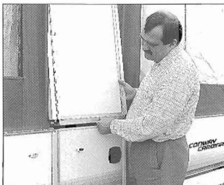
**20.** Close the bottom door and pushing the top door section upwards fit the channel at the base of the upper door over the lower door. Fit the plastic pegs in the upper door frame into the holes at the side of the bottom door.
