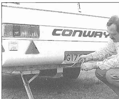
26. The spare wheel is mounted under the trailer at the back. It can be released using the corner steady brace.
