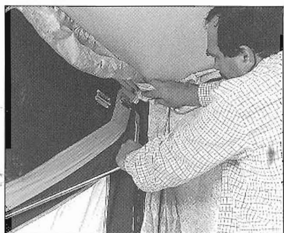
17. Push the bed end frame into the position and hold by fitting the first end of the roof support bar to slotted bracket. Repeat for each corner.
