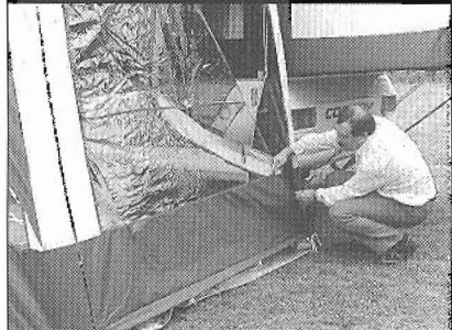
39. Unpeg and zip out the right hand awning wall.
