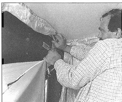
18. Fit the hooks at the front of the inner tents to the appropriate bracket. Once fitted the inner tents can remain clipped to the bed end frame, but must be unclipped from the front brackets before lowering your camper.
