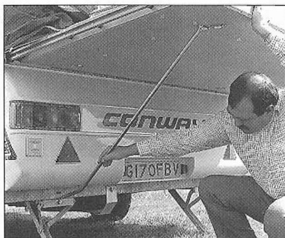
8. Fit the rear bed support bars to the slots cut into the chassis and to the bracket under the bed board. Repeat for the front bed.
