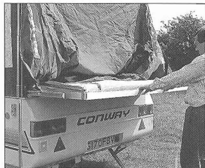
7. Pull out the rear bed until it reaches the bed end stop. Remove the bed support bars from under the mattress.
