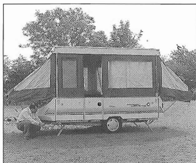
10. Ensure that the lower door is not catching or binding and then give each corner steady a further full one and a half turns.
