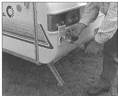
5. Slide up the winch socket cover and insert the winch handle.
