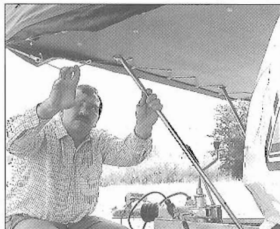
23. Fit the elasticated shock cord to the lugs fitted to the underside of each bedboard.
