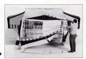
Pull down front of awning and locate gussets over centre and corner angles. (Care should be taken at this point not to snag the canvas or windows on the frame).
