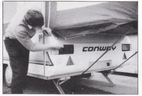
Elasticate the bed end underflaps onto the location buttons under the bed board.
