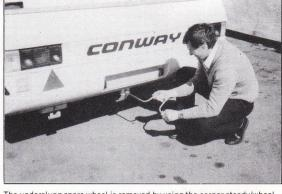
The underslung spare wheel is removed by using the corner steady/wheel brace to remove the retaining bolt, drop to floor then slide out spare wheel.
