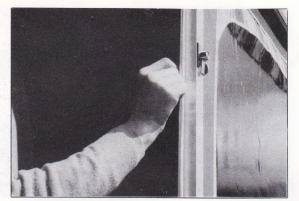
Release chrome clips on top door. Open door and step inside. Secure top door with turn buckles. To fit wall canvas to door, insert canvas hard edge into door channel by folding through 180° starting at the bottom, firmly press canvas into channel.
