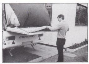
Pull out rear bed until it reaches the bed end stop and remove rear bed support bars from under each mattress.
