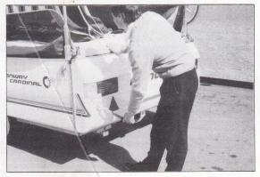
Slide up socket cover. Insert winch handle into winch socket.
