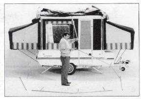
Hook centre roof pole into the eye on the front of the camper roof and then connect to the front 'A' frame.
