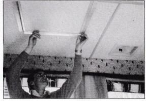
Unclip door from roof position, lower the door while you walk outside.
