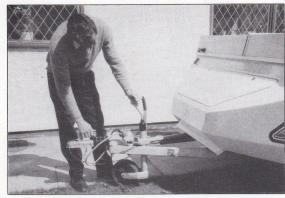
Park trailer in position required on site, fully brake trailer, unplug electrics, uncouple trailer from car. Level off trailer longitudinally by using jockey wheel. Level off sideways by means of proprietory caravan leveller or blocks. Wind down corner steadies onto wooden pads (i.e. no pressure).
