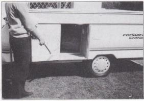
Lift roof corner by hand near door to avoid damage to draft seal on top of door. Open door and remove winch handle from interior of trailer.
