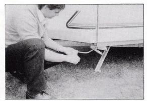
Finish off the four corner steadies by giving each steady a full  $\,1\%$  turns with the corner steady handle.
