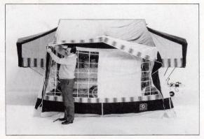
Fit the 3 short canopy poles between the main extension frame and front 'U' frame.
