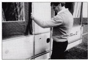
Close the lower door, take hold of top door section on both sides, lift against the spring hinge, lower top door onto bottom door, locating the oblong pegs into the mating holes at each side of the lower door and then pull the top door towards you.
