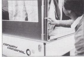
Turn handle clockwise to wind up roof, until the setting wire is taut, check periodically that the roof is rising equally.
