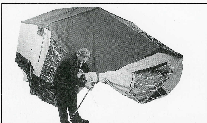
11 Pull canvas over front 'A' frame taking care to locate the eyelets over spikes on 'A' frame to avoid damage to canvas or PVC windows.
