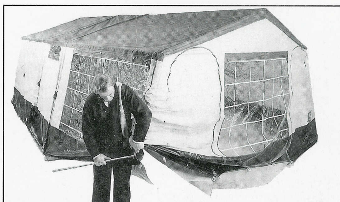
12 Spring together bottom section of frame legs and raise to full height.
