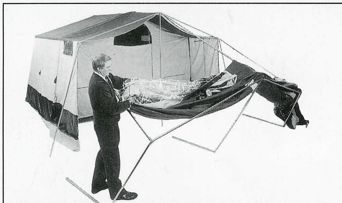
9 Unroll main extension canvas along roof poles.
