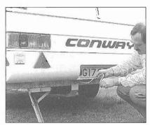
26. The spare wheel is mounted under the trailer at the bock. It can be released using the corner steady brace.
