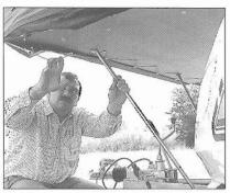
**23.** Fit the elasticated shock cord to the lugs fitted to the underside of each bedboard.
