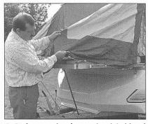
**9.** Fit the convas loosely around each bed board but do not secure with the elasticated cord at this stage.
