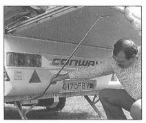
8. Fit the rear bed support bars to the slats cut into the chassis and to the bracket under the bed board. Repeat for the front bed.
