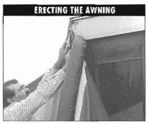
27. Remove the awning canvas from its bag and slide the white corded section through the awning channelling fitted to the camper roof.
