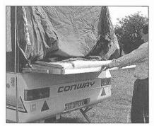
Pull out the rear bed until it reaches the bed end stop. Remove the bed support bars from under the mattress.
