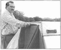
**29.** If the camper and the awning are being erected at the some time it is easier to fit the awning before the roof is raised.
