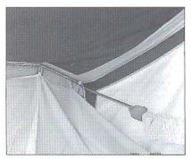
16. Remove the corner roof support bars from under the mattress, locate the open end over the plastic lug in the bed end frome.
