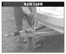
Apply handbrake and detatch trailer from the car. Ensure trailer is as level as possible using adjustment in the jockey wheel. On uneven ground aid levelling by using wooden blocks or other aids beneath the wheels.
