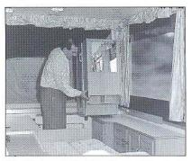
12. When vertical - slide the wardrobe across and into position on top of the cupboard units.
