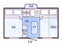
LAYOUT KEYFAFloor AreaBSBench SetteeFTFolding TableCCupboardFWFixed Window (Double Glazed)DBDouble BedOWOpening Window (Double Glazed)DBSDouble Bed/SetteeSLStorage Locker
