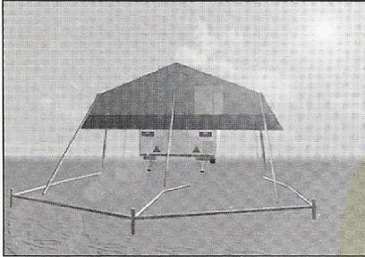
16. Take awning frame from bag and layout as shown. Assemble 'A' frame and hook in three roof support poles to main cabin.
