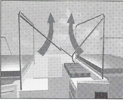
5. Release left and right hand centre 'A' frame ports from rubber retaining bands and button clip together at the centre.
