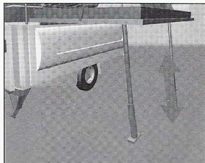
4. Adjust the heights of the bed legs if necessary to level bed.
