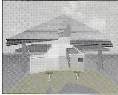
6. Pull canvas down from the roof at the front of the trailer. Open the door at the rear of the trailer.
