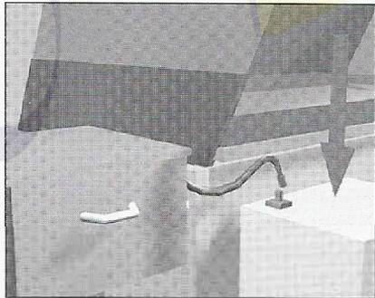
15. Click the gas pipe to the top of the cupboard making sure it is secure.
