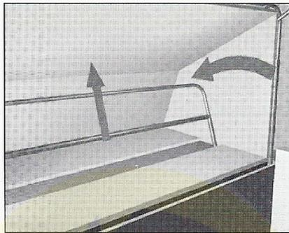
10. Fit left hand inner tent ensuring back rest support poles fit through slot in base of inner tent, extend frame and then hinge down flat and fit mattresses for use as a bed.
