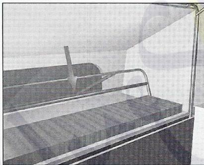
11. To convert left hand bed to a bench seat, hinge up back-rest support frame and lower top bar to short position. Fit the two support poles in brackets on the bed board and clip to bar. Reverse procedure to fold down.
