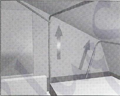
7. Step inside the trailer, push out bed end supports to first button clip and repeat for the central support uprights back and front.
