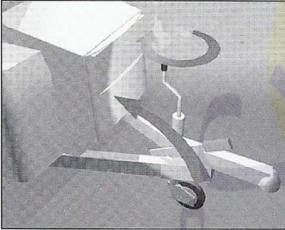
1. Apply handbrake and level trailer by means of jockey wheel.
