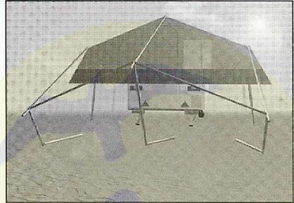
17. Fit front 'A' frame with legs 'broken' and connect 2 side roof poles to front frame.
