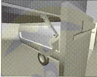
13. Swing the door support bar out and click in position. The door will click into the bar and hold firmly.
