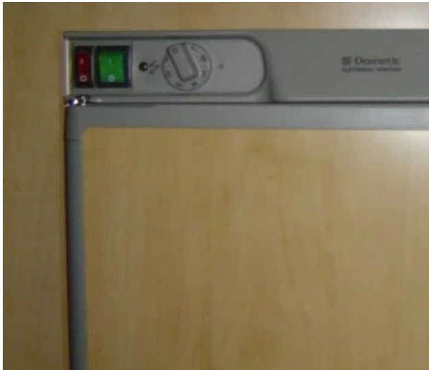
The 12V Switch, On A Fridge, Will Only Work Whilst Connected To A Car With The Engine Running
