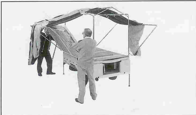
9 Fold over a bed board and mattress to each side. Check that each bed leg is securely located and adjust as necessary.
