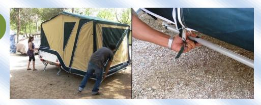
tep 8. For a better support use the included tubes for tensioning the tent.
