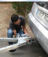
tep 2. Down the steady corners with the handle provided, until level the trailer Use the level included in the rear side.
