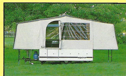
Extend telescope poles and secure canvas by press studs and Velcro.
