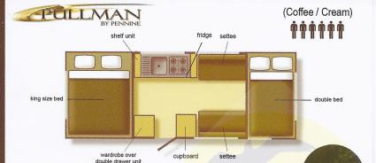
417cm Overall length 212cm Overall width 274cm Internal length Internal width 198cm Towing height 139cm Wheels 155 x 13"
