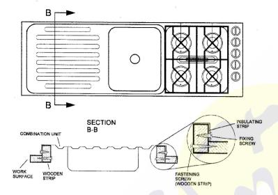
In the case of appliances that do not have grills fitted, the underside of the appliance must be shielded. It is recommended that the shield be fabricated from non-combustible material, but if the enclosure is manufacture from combustible material, then a minimum air space of 100mm (4") must exist between the material and the lowest part of the appliance.
