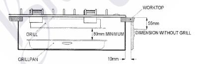
The grill compartment must have ventilation holes at the compartment floor level to prevent the accumulation of unburnt gasses.
