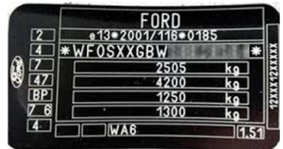
OK, so how does that help us? Well, the second number (GTW) tells us the absolute maximum that the car, trailer and full load are allowed to weigh. The top number (MGW) is the maximum that the car, alone, with full load, is allowed to weigh. Logically, therefore, the difference between the two is the maximum allowed weight that the car is allowed to tow. In the example above, the maximum towing capacity of the car is 1,695kg (4,200kg – 2,505kg).
