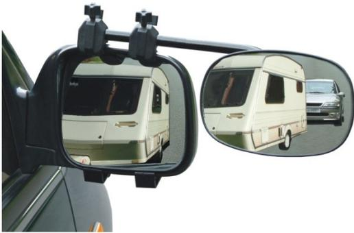
You must have an adequate view of the road behind you. If your caravan or trailer is wider than the rear of the towing vehicle, you will need to fit suitable towing mirrors.
