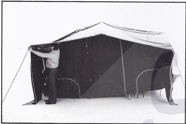
6 Fasten roof support poles to front 'A' frame.
